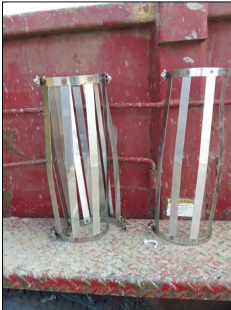
Centralizers are installed every 10 feet within the screened section, and every 80 feet along the rest of the casing.
